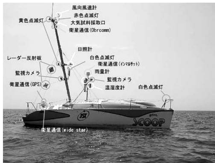
Fig. 9 Self Cruising Ocean Observation Platform (SCOOP). “Kan-chan” is a Japanese nickname.
